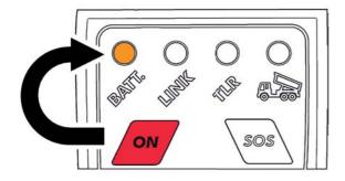
$\boldsymbol{\cdot}$  Light signal for battery status on the remote control
